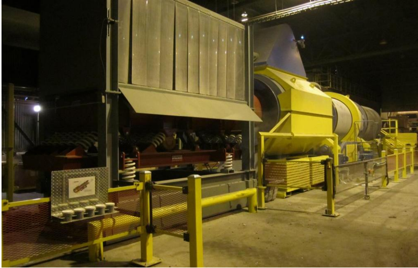
Figure1. Model RT 84 -2100 DIDION Metal/Dross Reclaimer
